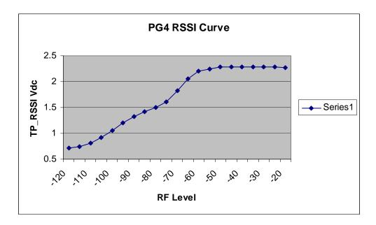
The microprocessor reads the RSSI level from an ADC several times a second when the PG4 is unmuted, to predict if a switch is necessary to avoid an audible dropout. Thresholds were calculated from the above RSSI curve.
